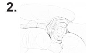
**2.** Flip cap over to access crystal retainer ring. Loosen ring by turning COUNTER CLOCKWISE.
