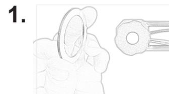
**1.** Obtain a copper Conflat™ gasket and place onto sensor head.
