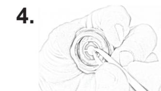
**4.** Use nonmetallic tweezers to adjust crystal position until crystal rests snugly in the crystal seat.
