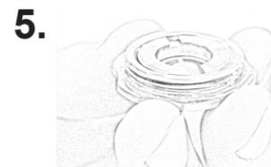
**5.** Place threaded side of retainer ring onto the corresponding threads of the sensor cap. Tighten by turning ring COUNTER CLOCKWISE using supplied tool.
