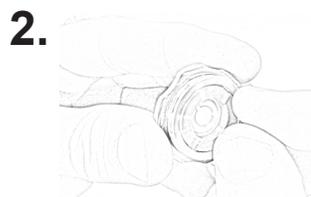
**2.** Flip cap over to access crystal retainer ring. Turn retainer ring COUNTER CLOCKWISE until loose.
