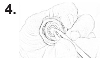
**4.** Use a nonmetallic prod to adjust crystal position until crystal rests snugly in the crystal seat.
