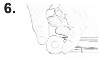
**6.** Place cap onto corresponding threads of crystal compartment. Turn COUNTER CLOCKWISE until secure.
